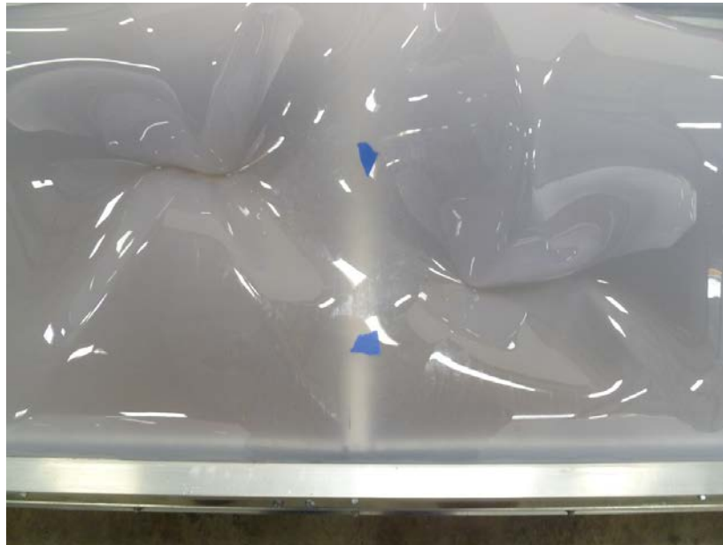
Photo No. 3 OSHA Safety Drop Test After Load Applied – Crease in Dome Ridges
